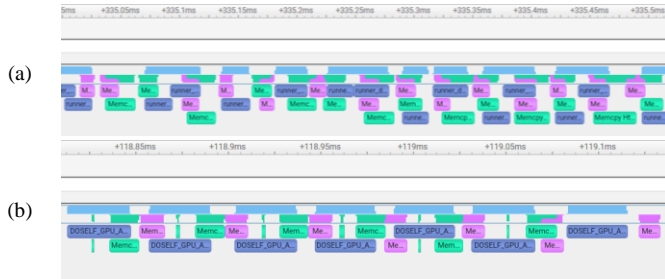
Figure 3. Profile for a GPU offload cycle on V100 with N_p=256^3 , S_p=2048 and S_b=512 . (a) Pair tasks. (b) Self tasks. Green, lavender and dark blue blocks represent CPU to GPU data transfer, GPU to CPU data transfer and kernels executing self and pair tasks, respectively.
