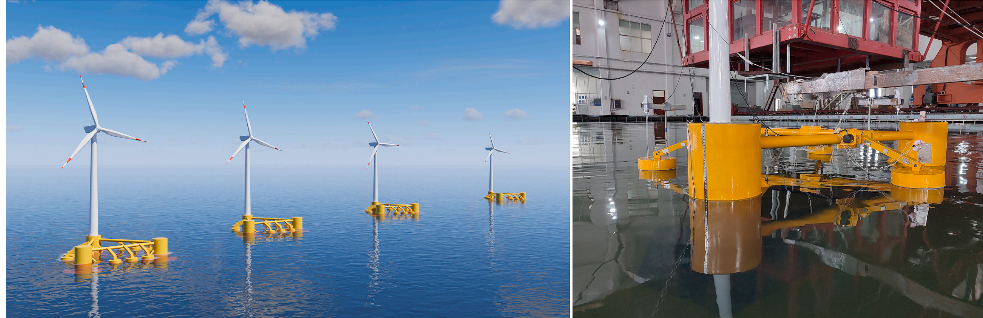
Rendered view of a wave-wind farm and a 1/40 experimental model of a wind-wave power system.
